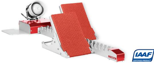
Footrest angle can be adjusted by 4 positions between 55° and 73°. Footrest can be moved horizontally within 16 positions spaced of 35.5 mm giving a maximum distance of 502.5 mm between front and back feet.
