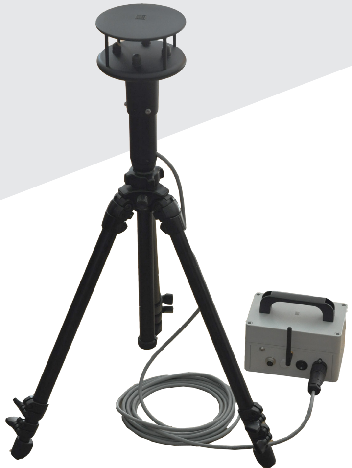
Wind meter on tripod with wireless transmitter
